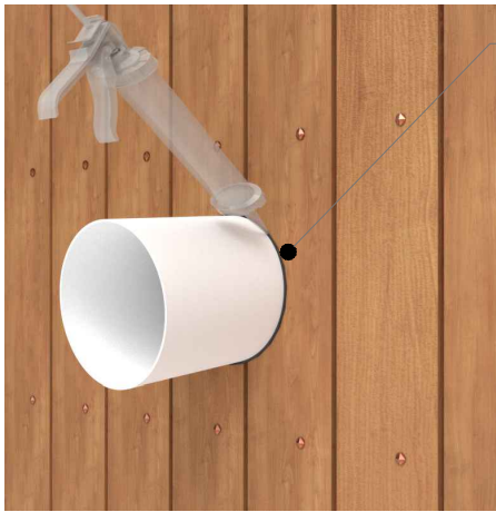
Continuous weather seal around pipe
